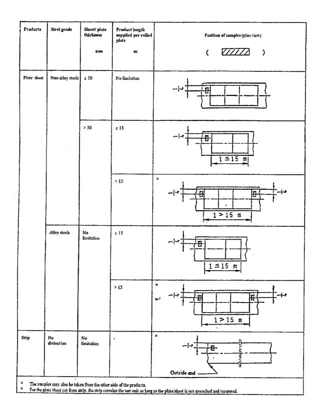
Figure 1 — Position from which the samples are taken
